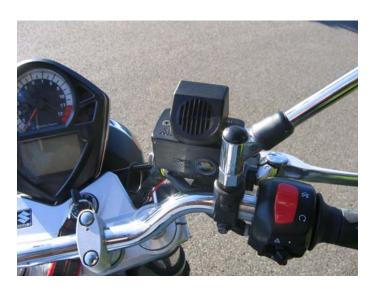
The Audicator has been designed to audibly alert the rider to the potential danger that the still active indicators present, when they are inadvertently left operating after the manoeuvre is completed.
